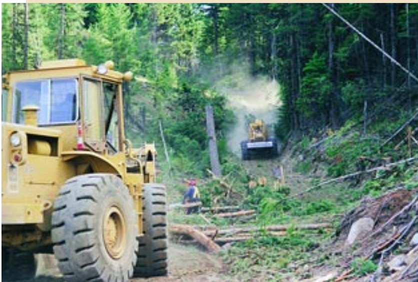
A grapple skidder hauls logs to the landing.
