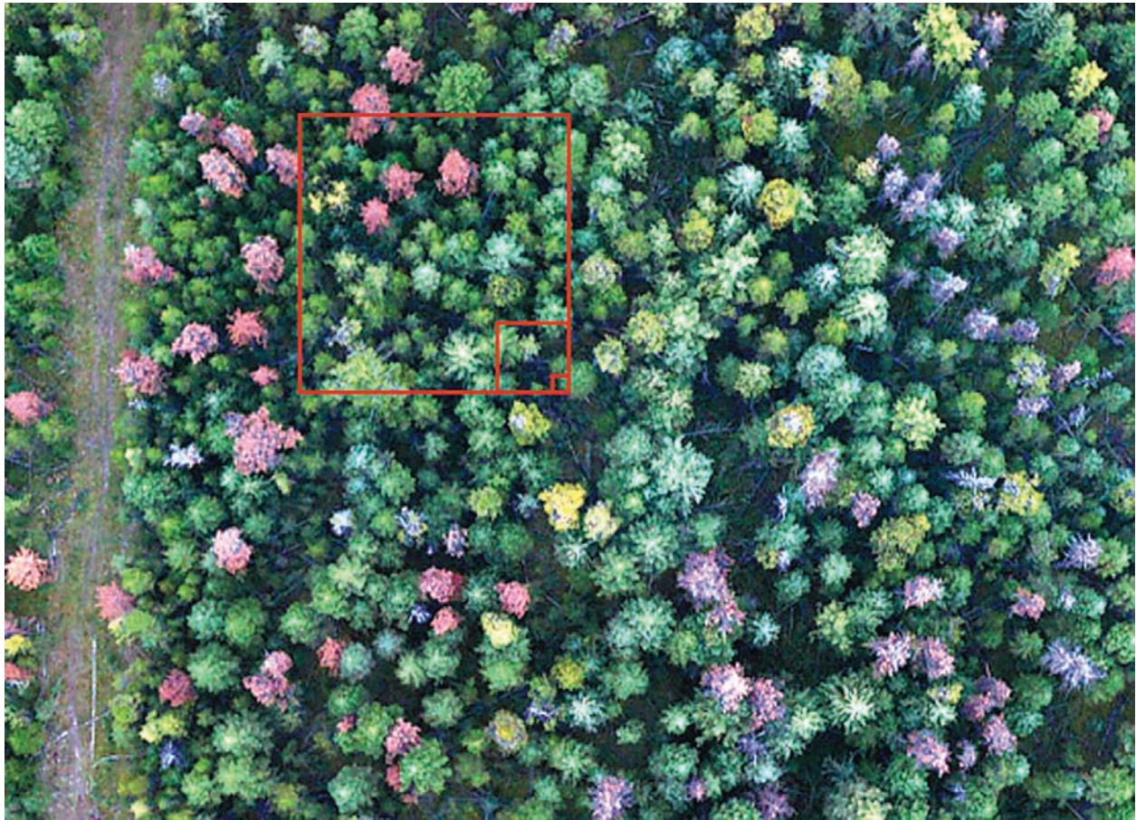
Figure 7. Illustration of information content of three common image spatial resolutions of 30x30 m, 4 x 4 m, and 1 x 1 m. Larger pixels tend to amalgamate a greater variety of stand elements. Underlying image is a true-colour digital photograph (from Wulder and Dymond 2004).
