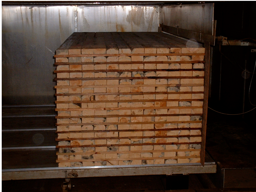
Figure 6: Dry kiln at Forintek Canada Corp. showing a load of post-MPB lumber
