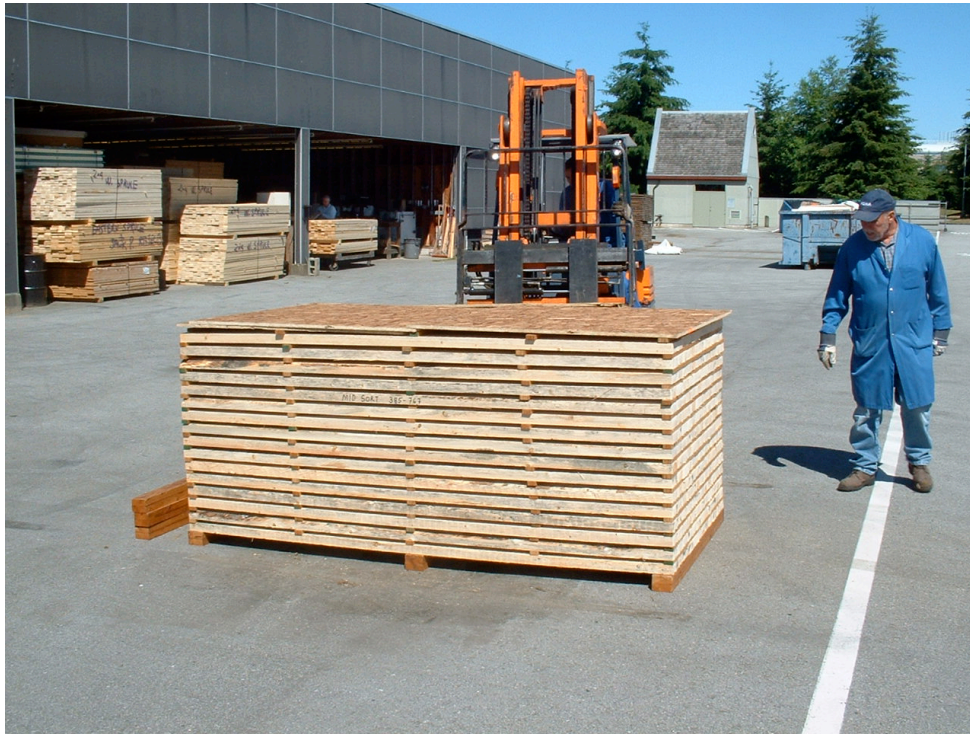
Figure 8: Air-drying in yard at Forintek
