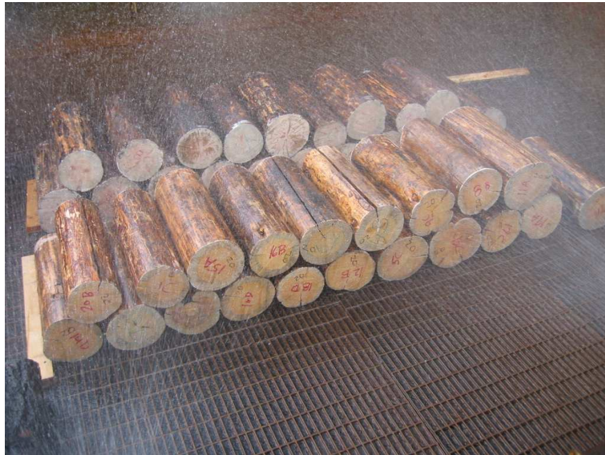
Figure 2 Water sprinkling on 2-foot MPB log samples
