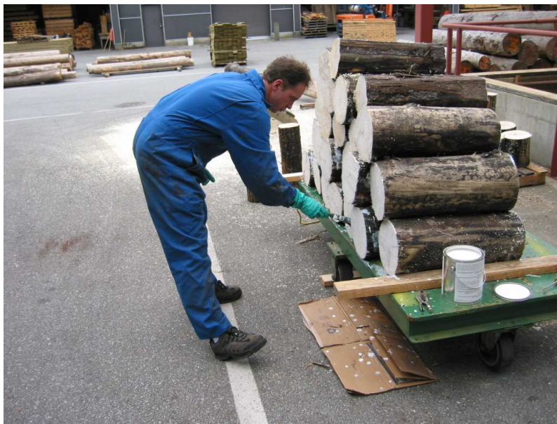
Figure 1 End-sealed 2-foot long samples
