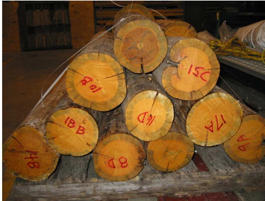
Figure 22 Checking in MPB logs prior to sprinkling
