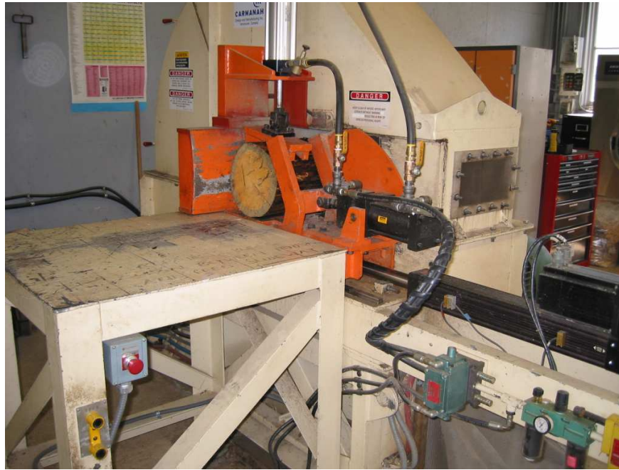
Figure 5 Carmanah laboratory drum strander
