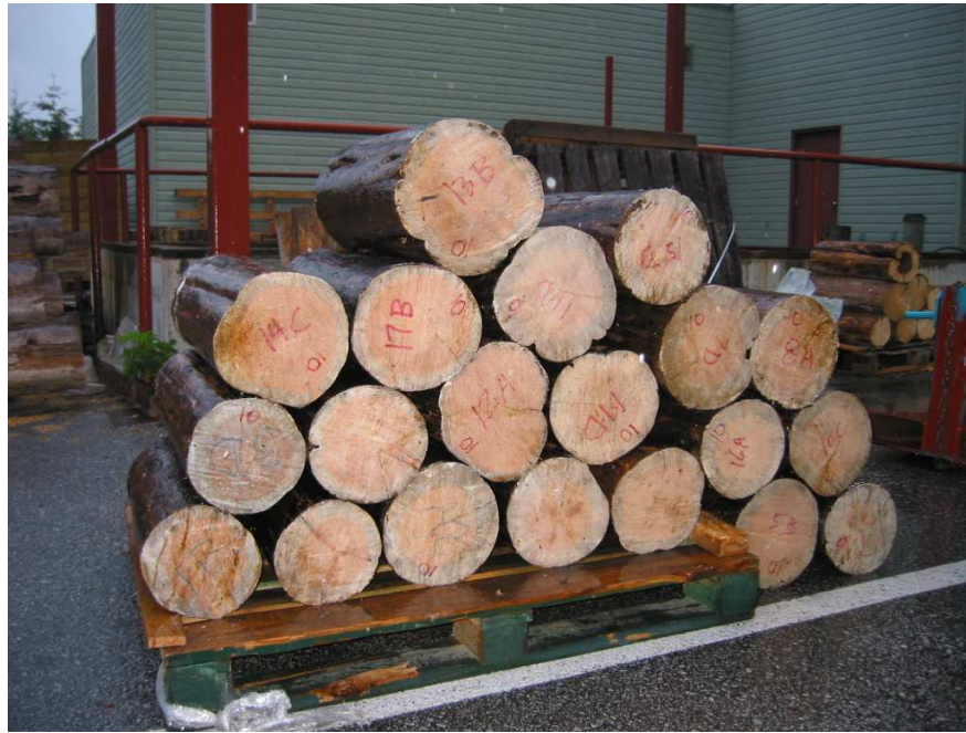
Figure 23 Checks in MPB logs have closed up after 10 days sprinkling
