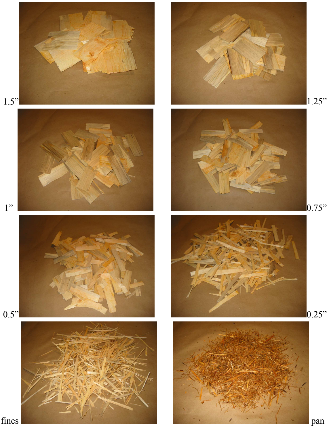
Figure 9 Screen fractions of different sizes from an MPB wood strand sample
