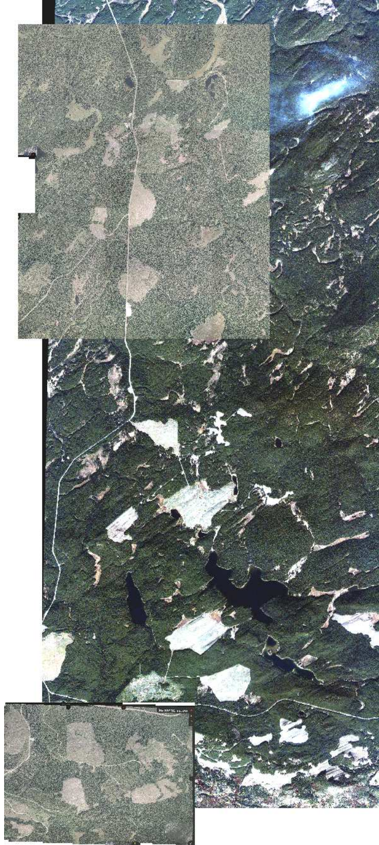
Figure 3. 1:20,000 colour aerial photography superimposed on IKONOS 4-m multispectral imagery. IKONOS imagery © Space Imaging LLC, all rights reserved.
