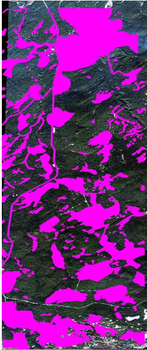
Figure 4. Exclusionary mask superimposed on IKONOS 4-m multispectral image. The areas under the mask were not included in the classification.
