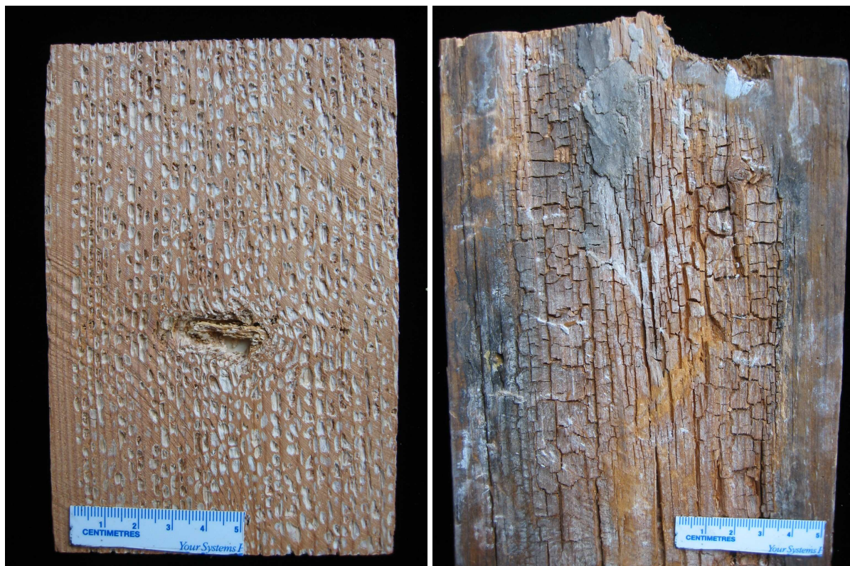
Figure 8. White pocket rot (left) and brown cubical rot (right).
