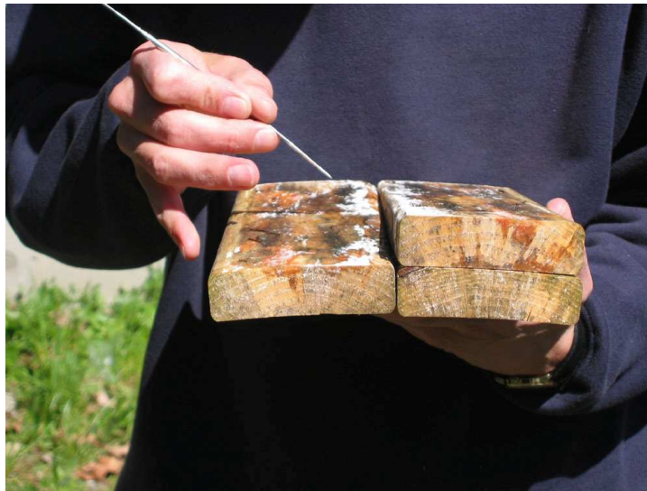
Figure 4. Probing a Scots pine sample for decay after 6.5 months of exposure. White-rot damage is visible on ends of component pieces.
