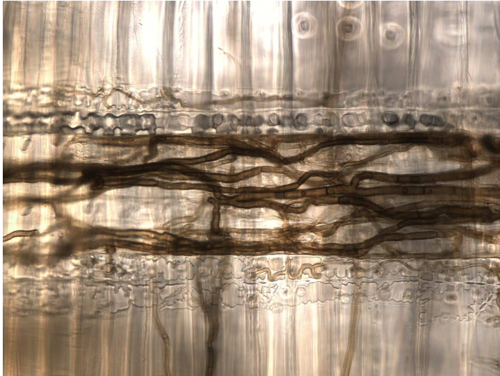
Threads of bluestain fungi in wood (Source: Paprican)
