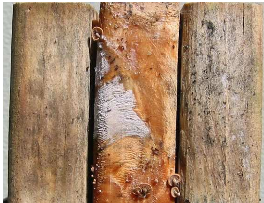
Figure 5. Fruiting body of wood-decaying basidiomycete fungus on Scots pine sandwich unit after 6.5 months of field exposure.
