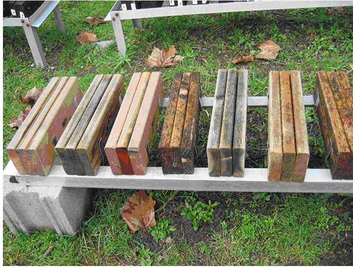
Figure 3. Close up of typical sandwich test units four months after installation. The Scots pine units are fourth and seventh from the left.
