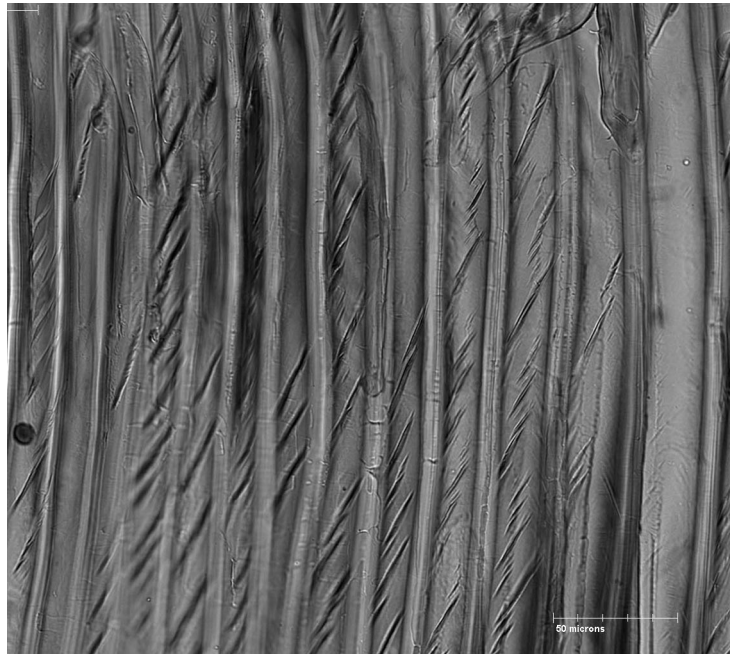
Figure 6. Soft rot damage caused by Chaetomium globosum in pine showing characteristic orientated diamond shaped cavities in cell walls (400x).
