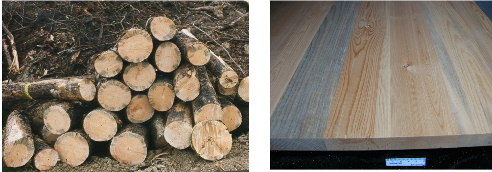
Figure 1. Bluestain showing wedge-shaped patterns in lodgepole pine sapwood (left) and as revealed in edge-glued lumber panel (right).
