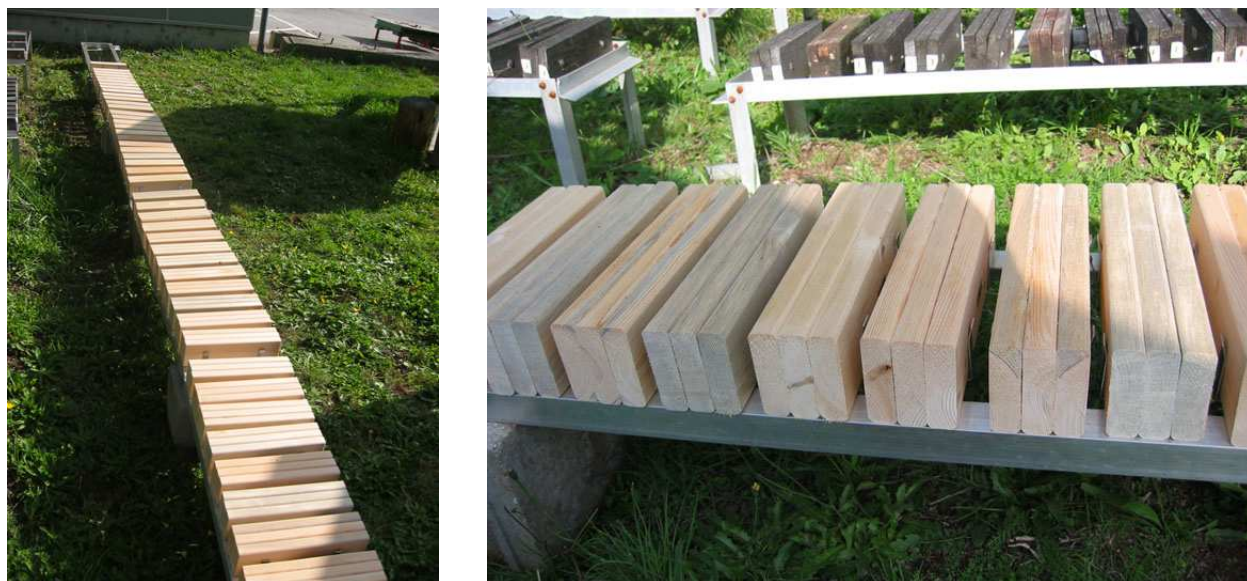
Figure 1. General appearance of sandwich tests in field exposure at set-up.
