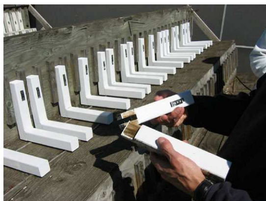
Figure 6. Appearance of typical bluestained L-joint after 6.5 months of field exposure.
