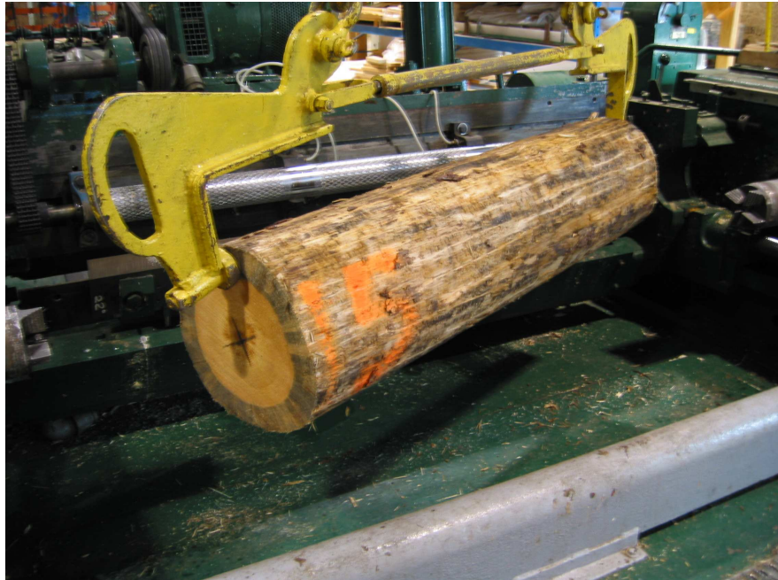
Figure 8: Scale-up peeling test with 4-ft (1.2 m) lathe
