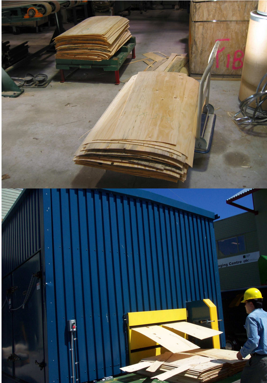
Figure 18: Drying MBP veneer with pilot-scale dryer
