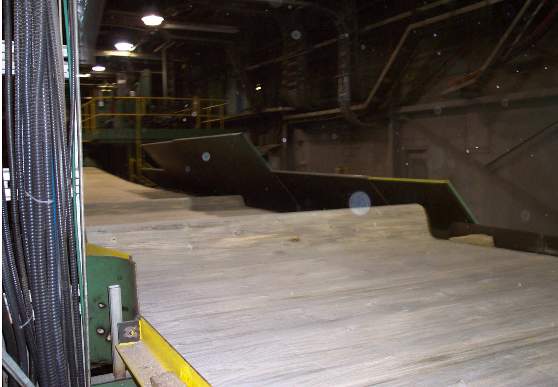
Figure 9: Ribbon of MBP veneer coming off the 8-ft (2.44 m) lathe
