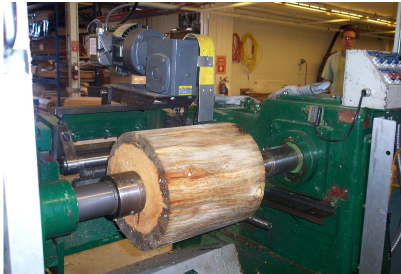
Figure 7: Peeling veneer with 15" (38 cm) mini-lathe
