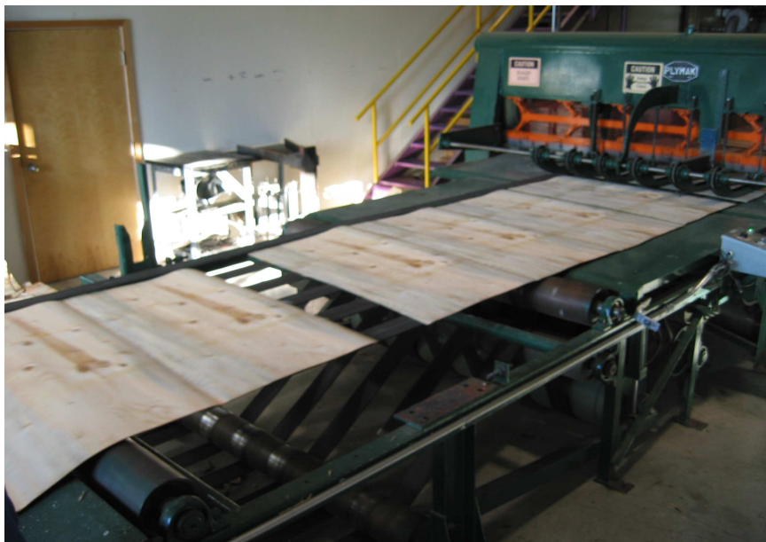
Figure 15: Veneer ribbon coming off the 4' (1.2m) lathe
