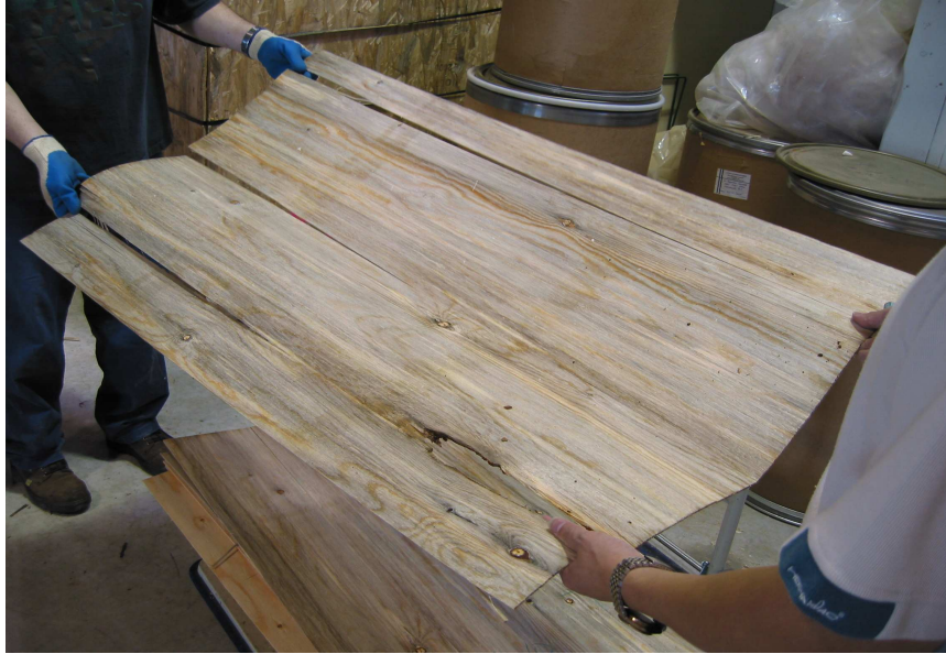
Figure 16: Splits in the MBP sap veneer sheet
