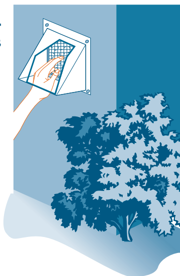
FIGURE 6 Checking exterior inlets and outlets
