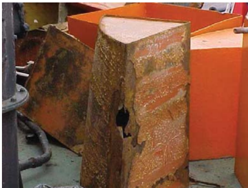
Corroded Lifeboat Buoyancy Tanks
