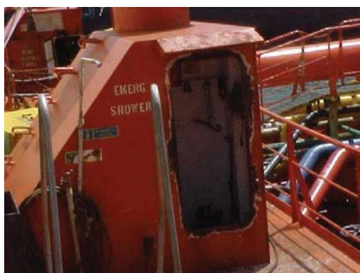
Watertight door missing
