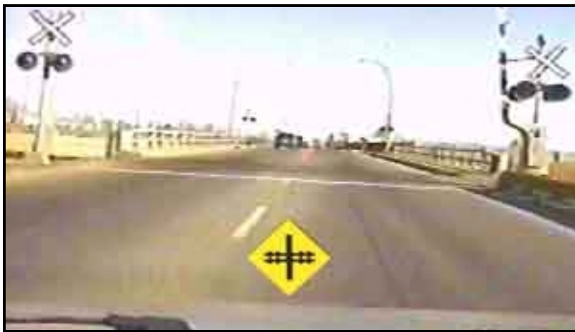
Figure 5.1 Head-up display of in-vehicle train warning used in Chugh and Caird (1999).
