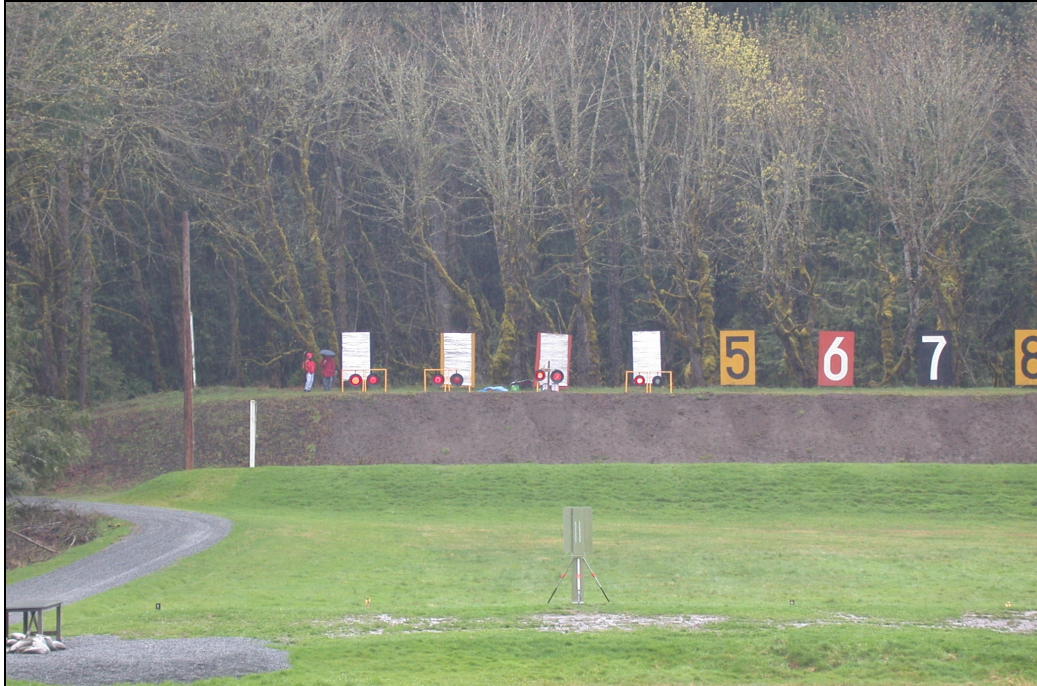
Figure 38 Test Set-up with Reflective Sheets Behind the Lights
