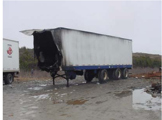
Trailer fire damage
