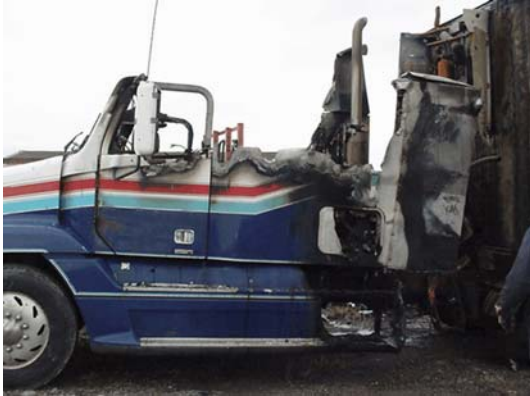
Tractor fire damage
