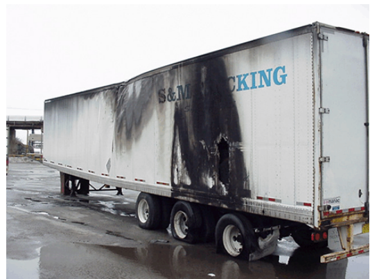
Drop trailer fire damage
