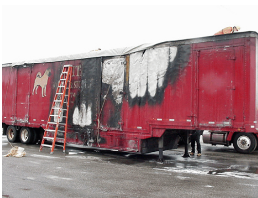
Moving and storage trailer fire damage
