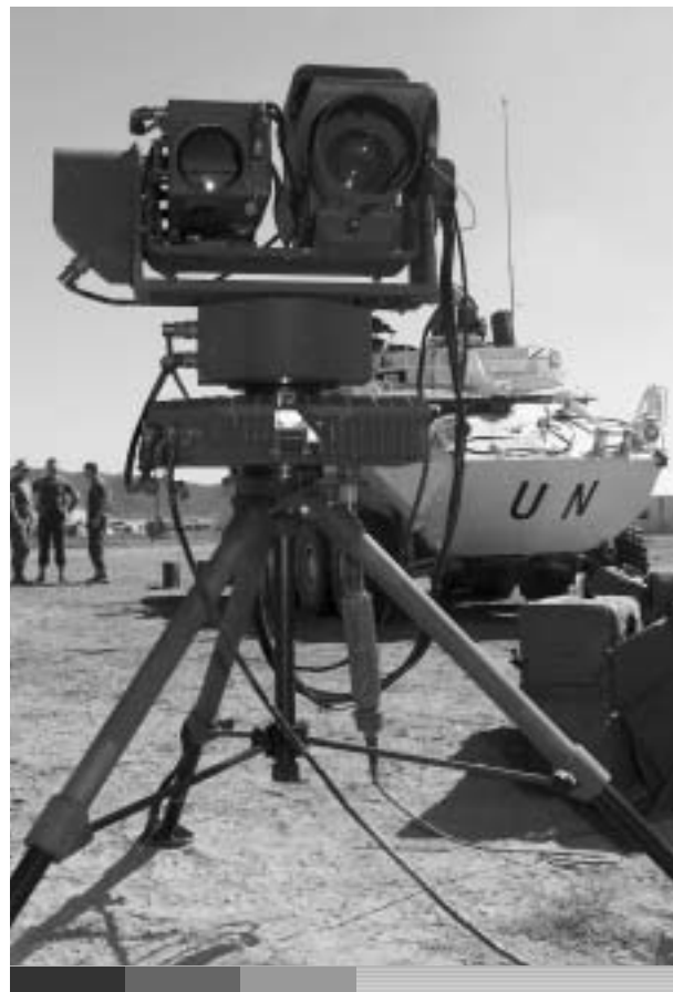
Coyote surveillance system camera.
