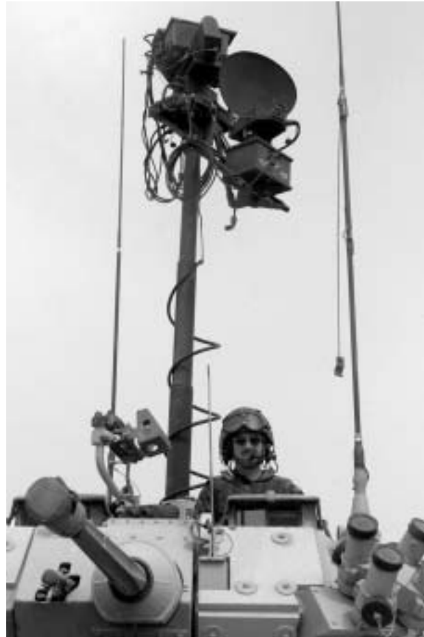
Mast-mounted radar assists in C2.
