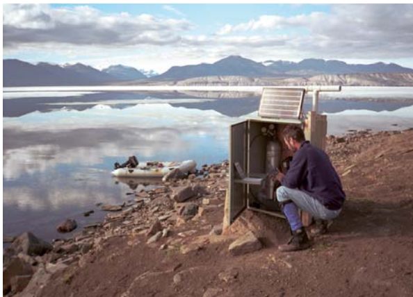
Hydrometric stream gauging station. Ruggles River at outlet of Lake Hazen, Quttinirpaaq National Park.
