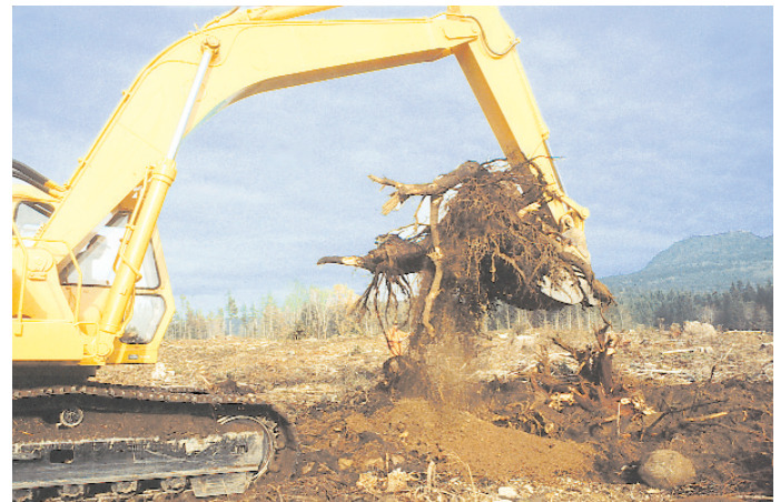
Removal of a root-diseased stump with an excavator.
