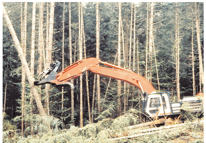
A whole, root-diseased tree is push-felled with an excavator.
