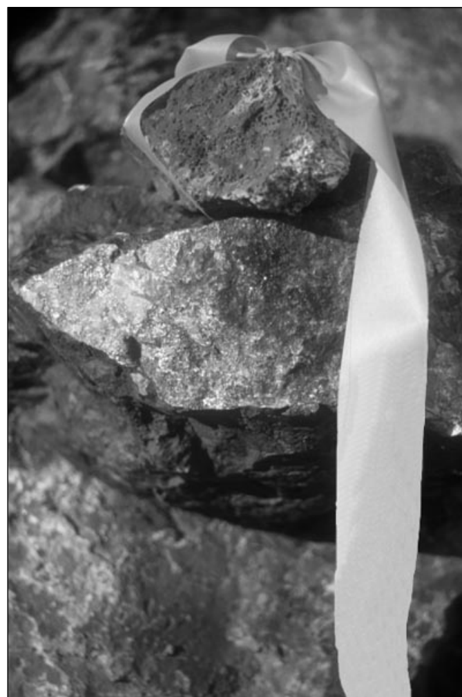
Figure 3. This sample of weakly brecciated pink to beige chert with disseminated and fracture-controlled chalcopyrite assayed 1.92% Cu.
