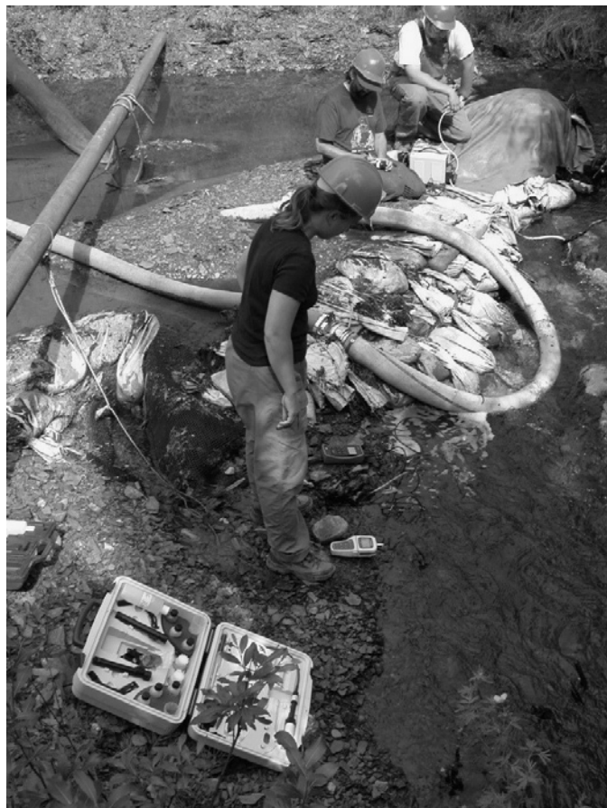
Figure 2. Authors sampling at location BC05-02 next to the pump house. In the foreground, pH, DO and SEC measurements are being taken. In the background, the samples are being collected.
