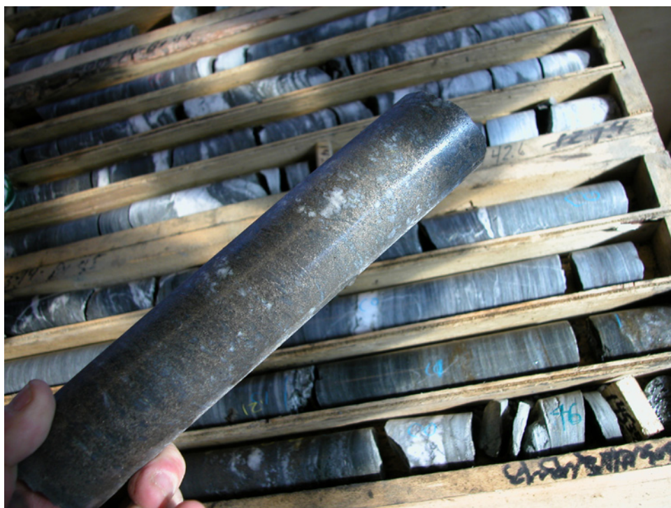
Figure 11. Gold-bearing semi-massive pyrrhotite in core from the McQuesten property.
