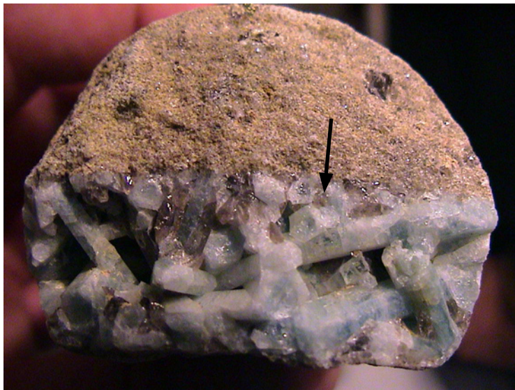
Figure 23. Light blue beryl crystals in drill core from the Goddess (Pluto) property.
