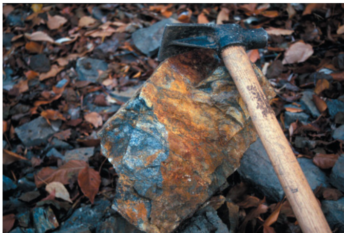
Figure 2. Silicified and brecciated siltstone such as this, assayed up to 24 g/t Au.
