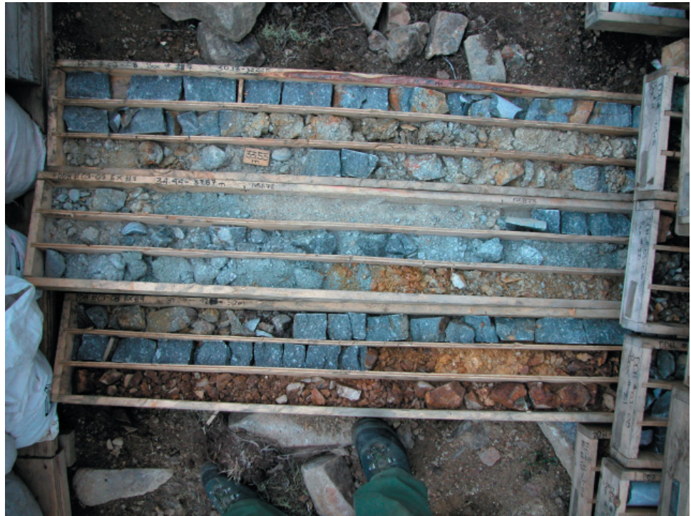
Figure 7. Faulted quartz monzonite in Hole 8 on the Ice property assayed 1.12 g/t Au from 31.0 to 42.3 m.
