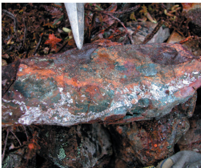
Figure 8. Pyrrhotite skarn mineralization from the Mahtin property typically assayed between 1 and 4.3 g/t Au.
