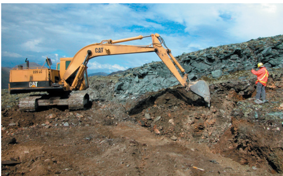
Figure 20. Surface bulk sampling under close geological control at Regal Ridge.
