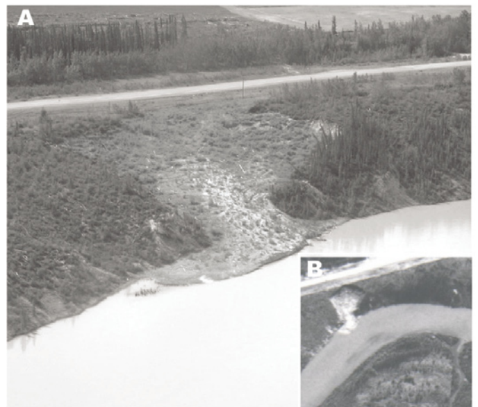
Figure 11. (a) Oblique aerial photograph taken in 2003 of Takhini River retrogressive ground ice slump. (b) Inset aerial photograph taken in 1987 of Takhini River retrogressive ground ice slump.
