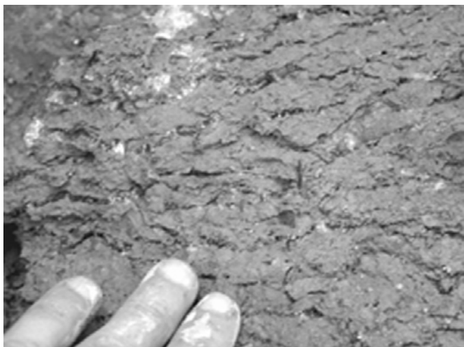
Figure 5. Photograph of frozen soil with stratified ice veins (1-3 mm thick) from Location B, the unburned forest site in Figure 4.
