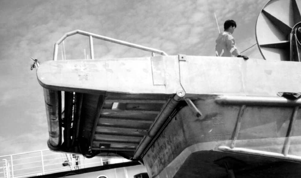
Stern of Cap Rouge II showing solidly constructed stern ramp extending beyond the transom
