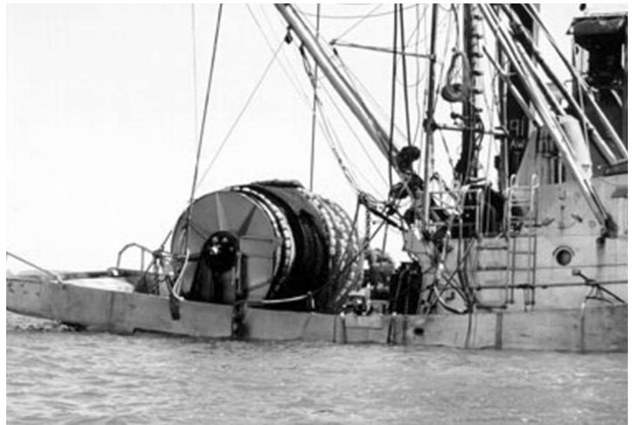
Working deck of Cap Rouge II showing west coast salmon seine net wrapped on net drum
