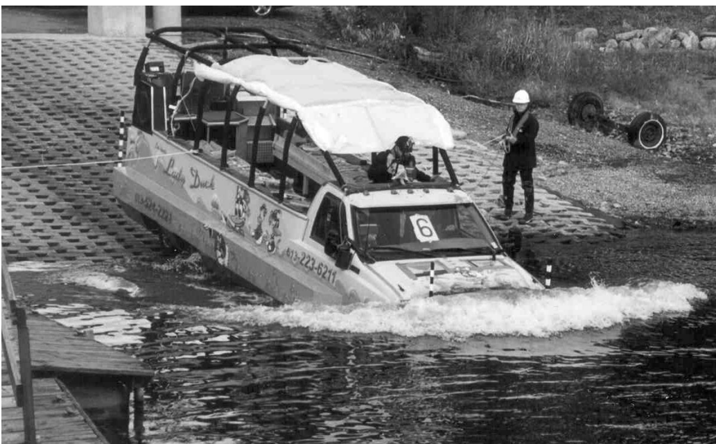
Vehicle launched at 8 km/h, visor submerged by approximately 25 mm
