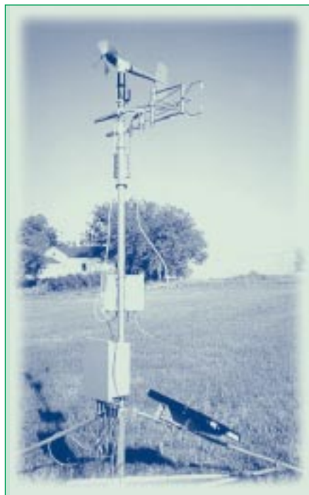
Monitoring equipment used to measure toxic fluxes between the soil and air.
