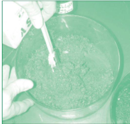
Researchers create a “chocolate mousse” in the laboratory at the Environmental Technology Centre to study the process by which water-in-oil emulsions form during oil spills at sea.
