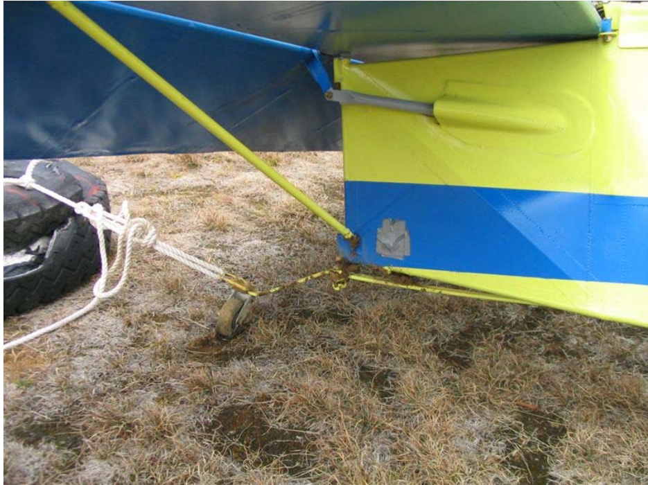
Photo 5: Tail leaf bracket damaged
