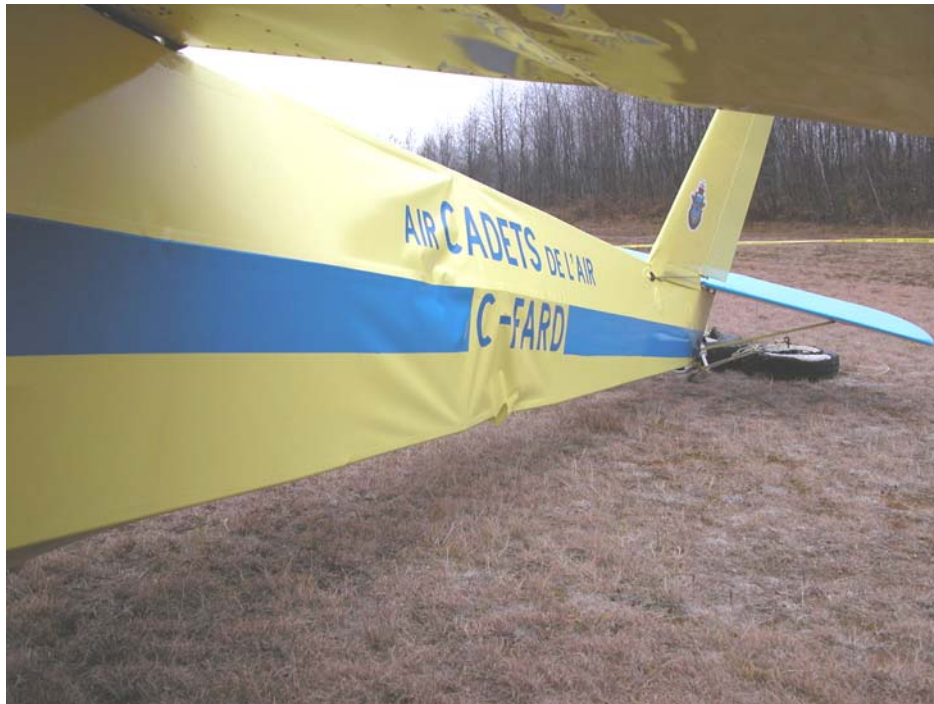
Photo 4: Left Wing and Fuselage damage
