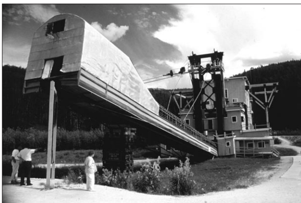
Dredge No. 4 buried in silt on Bonanza Creek; stacker in foreground
