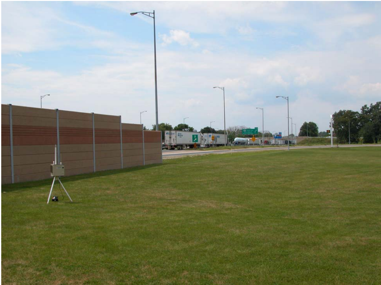
Figure 43: Monitoring truck impacts downwind of Highway 402 wall in Sarnia
