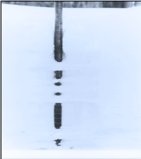
Several crusts have been penetrated by the "pogo stick" gauge in this carved-away snow drift. Photo- P. C. Smith.
