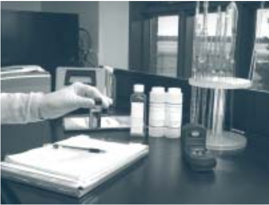
Conducting chlorine residual test using a portable analyzer
