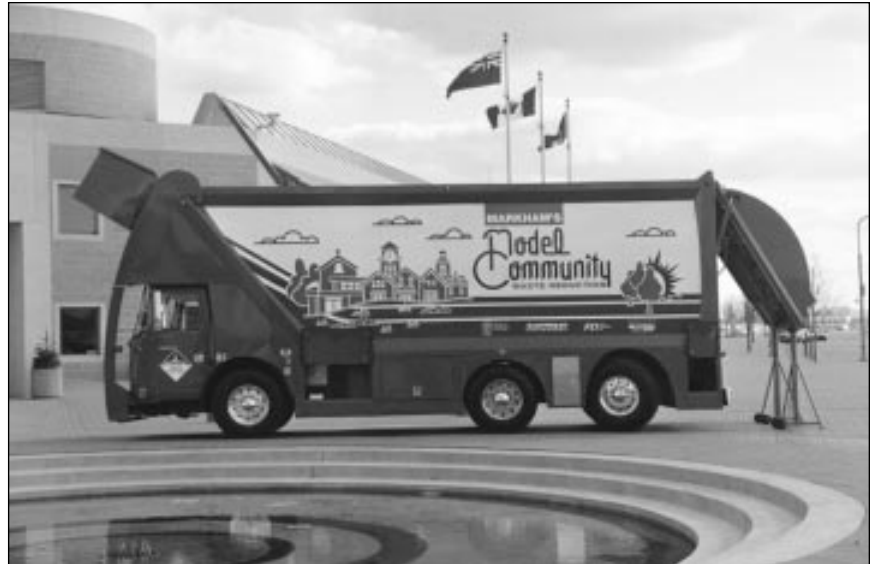
Fiba Canning’s Refuse Collection Vehicle with Regenerative Brake Energy System
