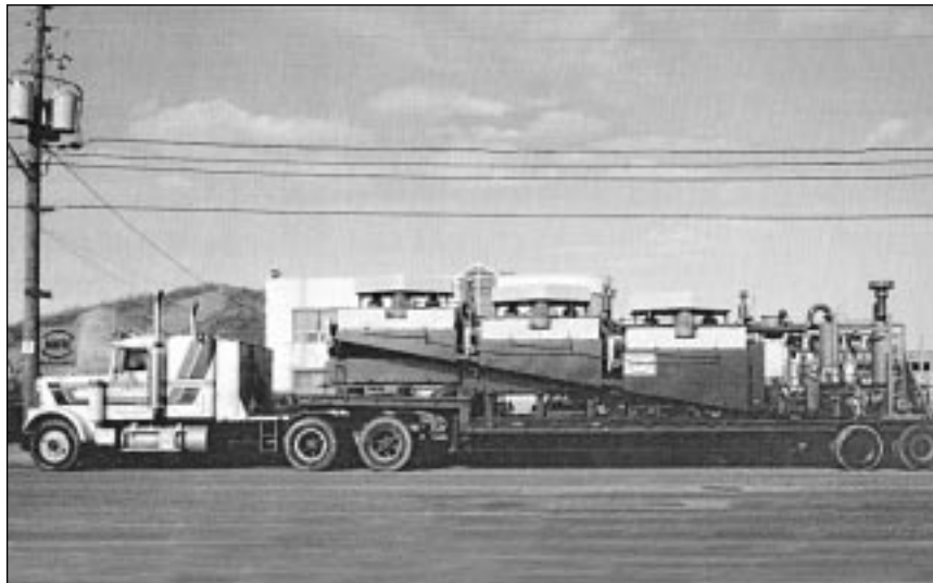
Flotation module of 50 ton per day soil wash pilot plant
