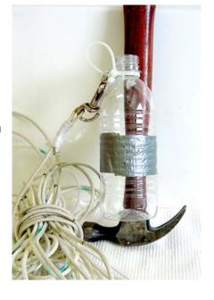
from the bottom. You will need to collect one sample to fill the PET jar and a second sample to fill the two test tubes.
