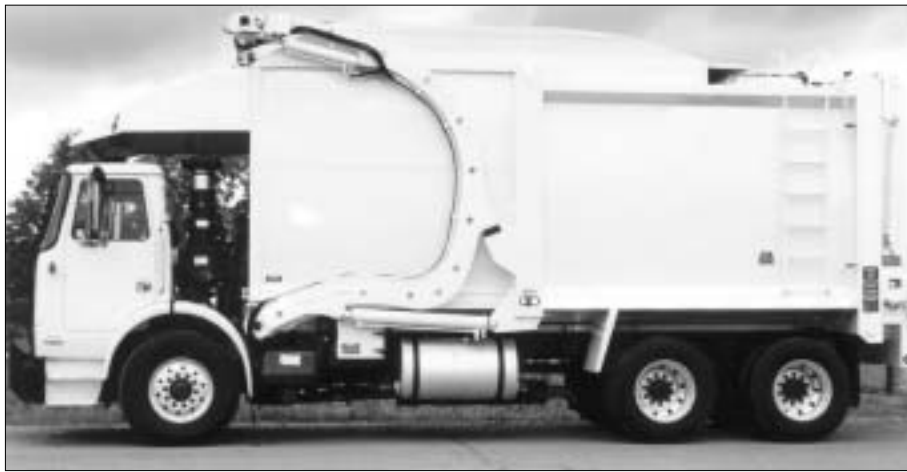
Figure 11 - Front-loading compacting equipment (loading forks extended)
