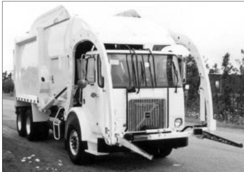
Figure 11 - Front-loading compacting equipment (loading forks extended)
