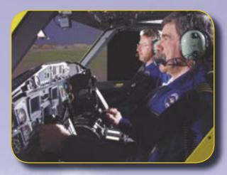
The FTD reproduces a CL-415 air tanker cockpit. The crew watches the action on a 180° screen.
