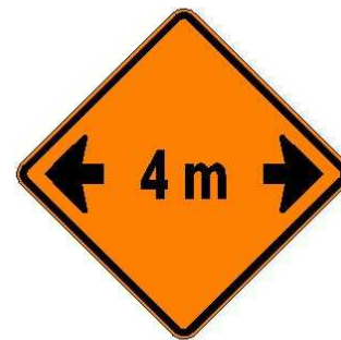
Sign T-180 Horizontal clearance
