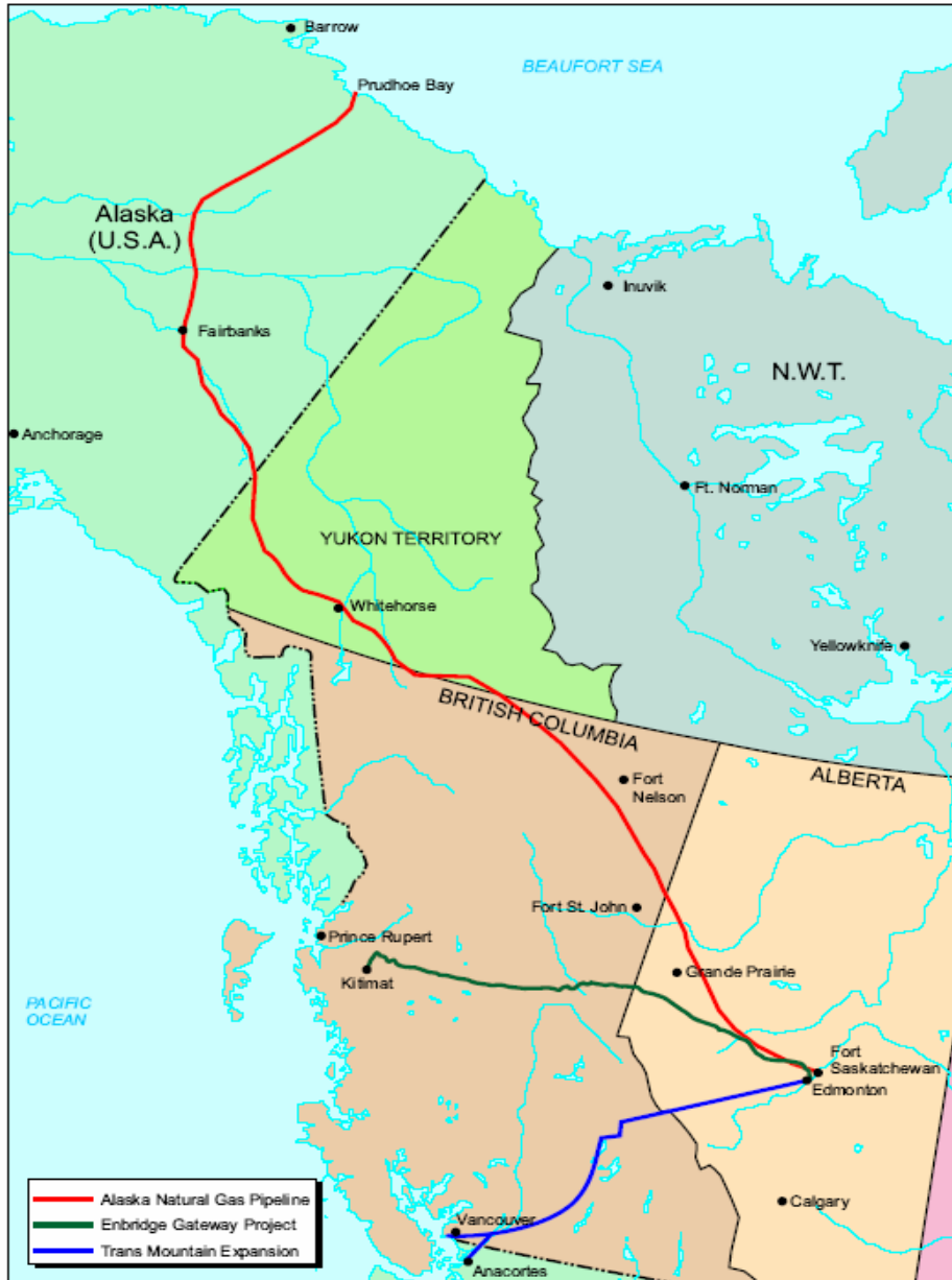
Figure 3 – Proposed Major Pipeline Projects in B.C.
