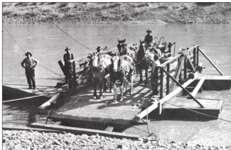
Big Bar reaction ferry on the Fraser River in 1920. Over the years, the basic design of this type of ferry has not changed. In 2001 there were still six in use throughout the province.
