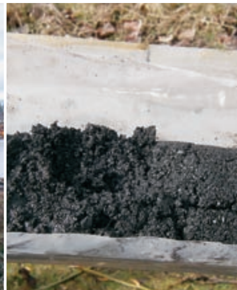
Ladysmith Harbour – Soil sample from drilling comprised of waste coal material
