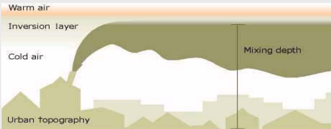
Figure 3: Diagram of a Temperature Inversion. The warm layer of air on top of the cold layer creates an inversion layer that traps emissions close to the ground. Graphic courtesy of Environment Waikato, Government of New Zealand.
