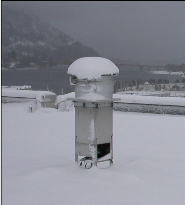
Figure 3 -- High-volume (Hi-Vol) manual sampler on the roof of the government building collects a sample over a 24-hour period every sixth day
