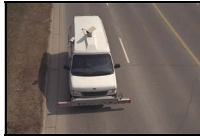
Automated Distress Survey
