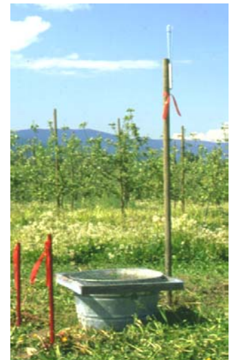
Figure 5 Manual Rain Gauge Location
