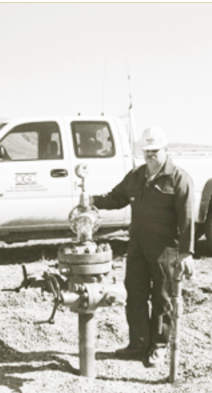
Bruce Cazes, Manager of Drilling and Completions, inspects a CBM test well in Hudson's Hope, BC
