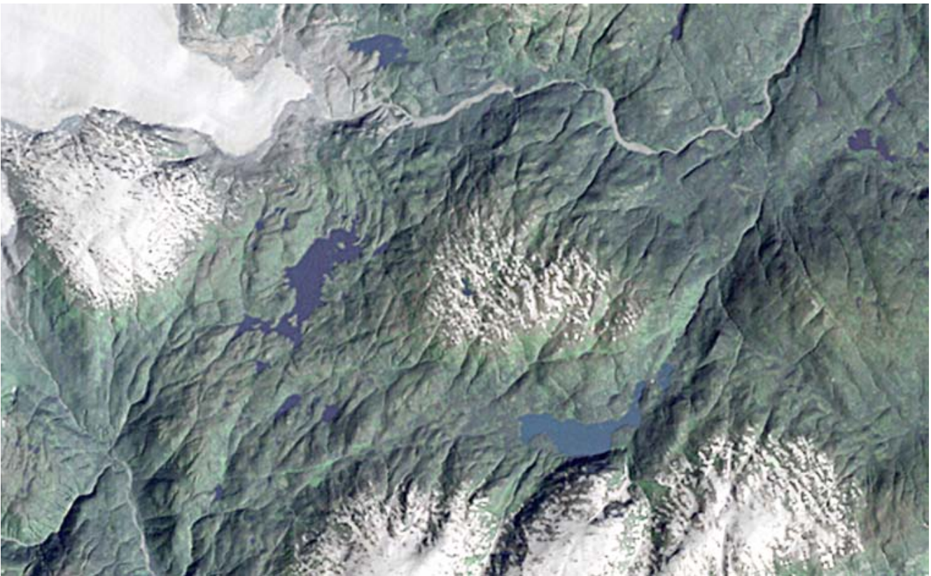
Figure 5. Enhanced Landsat image formed from the fusion of hillshaded image and natural colour image.
