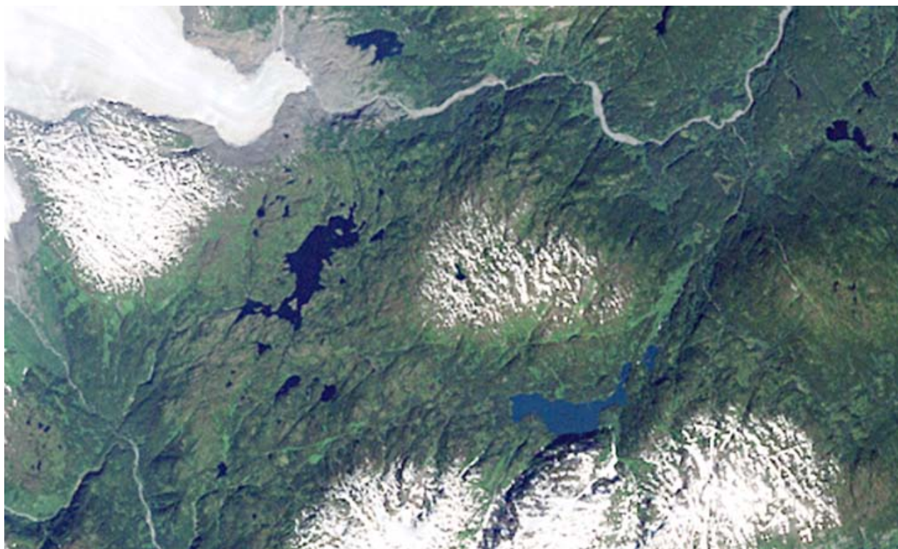
Figure 3. Natural Colour Landsat image based on bands 3, 2, 1 as red, green and blue, respectively.
