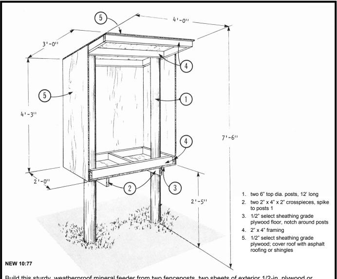
Build this sturdy, weatherproof mineral feeder from two fenceposts, two sheets of exterior 1/2-in. plywood or Aspenite, 32 ft of 2 x 4-in. lumber and some asphalt roofing. For better durability, use pressure-treated posts and galvanized nails.
