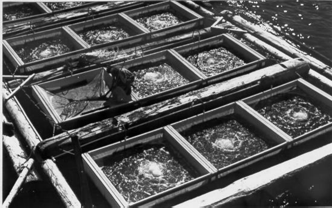
Figure 1. Photograph of the Floating Algal Culture System (F.A.C.S.) used as the primary screening apparatus.
