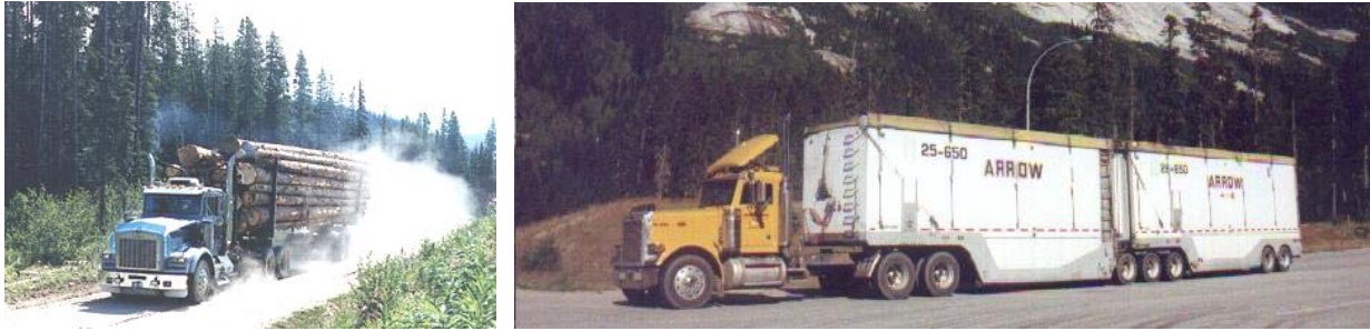
Figure 2.3.2 7-Axle Logging Trucks Are Used in BC (left), as well as Chip Trucks (right)
