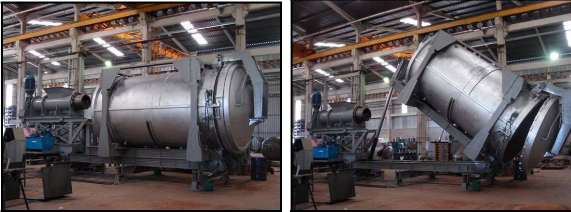
Figure 4.2.8 Prehydrolysis Reactor (a) Horizontal and (b) Cellulignin Dumping Position
