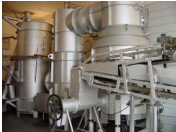
Figure 4.6.4 A Gasifier by Vidir Machine Inc. This Stationary Gasifier Unit Could Easily be Converted Into a Mobile Unit.
