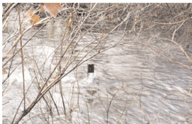
The Black Creek Recovery Project involves the collection of hydrology and temperature data. Pictured above is a gauge on Black Creek during high-flow season.
