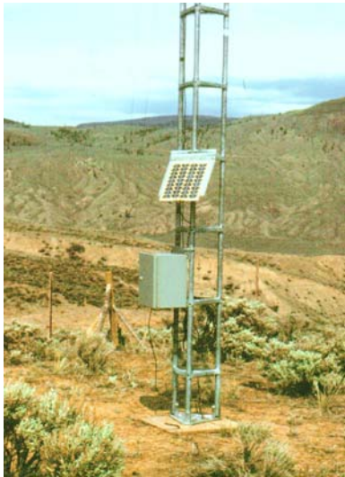
Solar-powered Data Collection of Wind Speed
