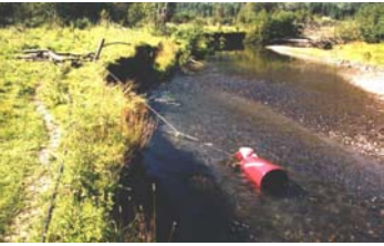
5b Anchored to a Streamside Post
