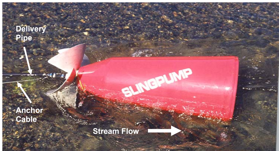
Figure 2 Sling Pump Operating in a Stream
